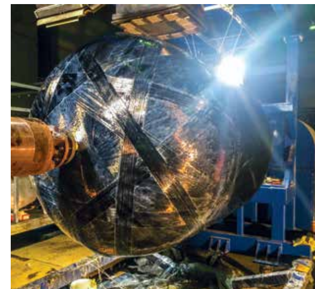
To achieve EU certification, Omni Tanker had to go through a so called 'Burn Fire Test' in Germany. As part of it, the tank is subjected to a full engulfment fire of around 850-1000°C for 30 minutes and must remain leak free after the test.
